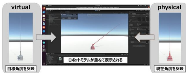
Figure 3 Explanation of the Unity screen while operating the robot
