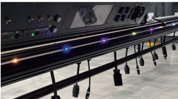
Figure 5: Illuminated display of installation location
