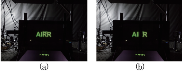
Fig. 3 Aerial image (a) with small gap (b) with large gap.
