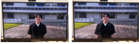
Fig. 6: Stereo Images captured from the position of both eyes of a stereoscopic video displayed in autostereoscopic 3D on the receiving side.
